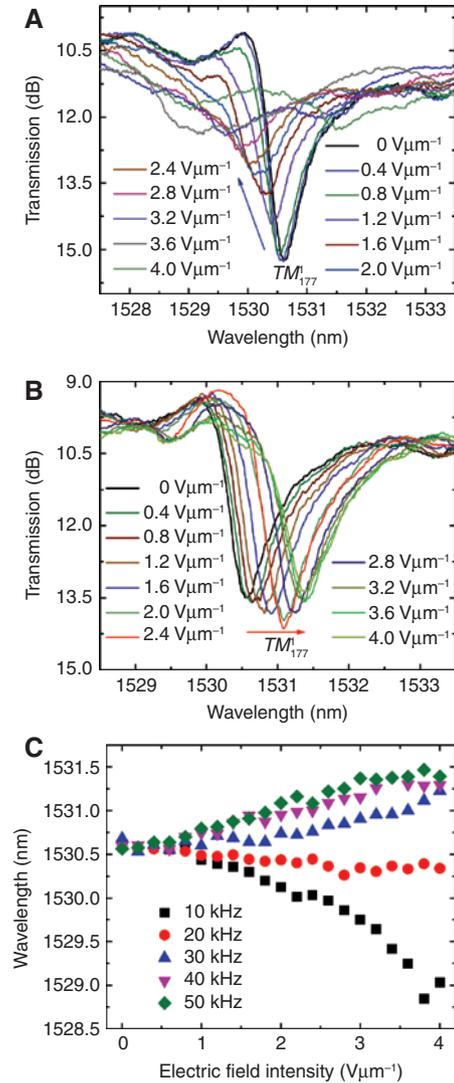
**Figure 7:** Transmission spectra of the grapefruit-MOF-based microresonator filled with DFLC-2 under the applied electric field at (A) 10 kHz and (B) 50 kHz, respectively. Arrows in these figures indicate the spectral shift direction with the increment of the applied electric field intensity. (C) WGM resonance wavelength shift as functions of applied electric field for different AC signal frequencies.
