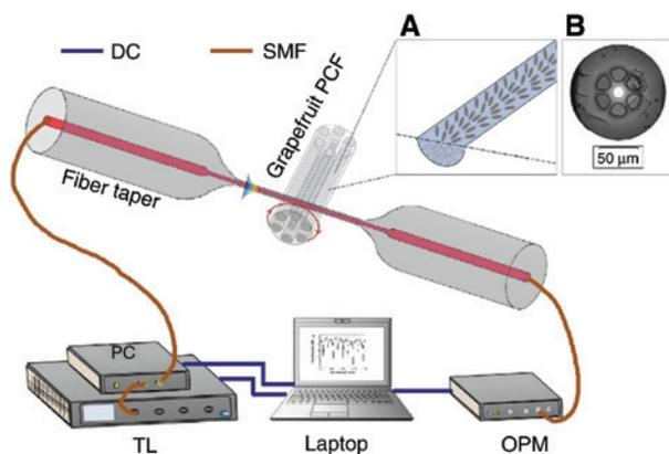
**Figure 1:** The experimental setup for performance testing of the proposed MOF-based microresonator integrated with LCs. DC, Data cable; grapefruit PCF, grapefruit photonic crystal fiber; PC, polarization controller; OPM, optical power meter; SMF, single-mode fiber; TL, tunable laser. Insets (A) and (B) show the schematic orientation of LC molecules in the grapefruit MOF and the cross-sectional microscopic grapefruit MOF, respectively.
