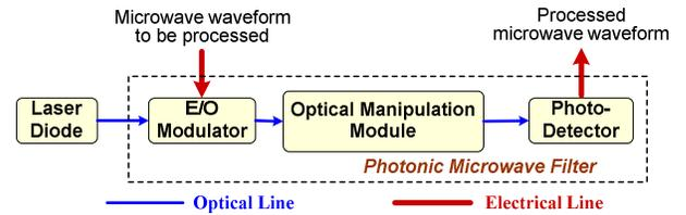
Figure 6. General diagram of a photonic microwave filter for microwave waveform processing. E/O: electro-optic.
