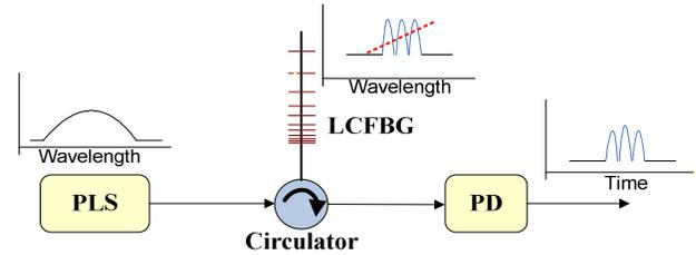
Figure 3. Schematic diagram showing a microwave arbitrary waveform generator using a single LCFBG. PLS: pulsed laser source, LCFBG: linearly chirped fiber Bragg grating, PD: photodetector.
