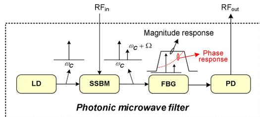
Figure 7. Schematic of a microwave waveform processing system for chirped microwave pulse compression. LD: laser diode; SSBM: single sideband modulator; FBG: fiber Bragg grating; PD: photodetector.
