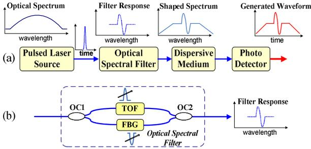
Figure 2. (a) Schematic diagram of a microwave AWG system based on optical spectral shaping and dispersion-induced frequency-to-time mapping. (b) An optical spectral filter designed for ultra-wide band pulse generation. OC: optical coupler, TOF: tunable optical filter, FBG: fiber Bragg grating.
