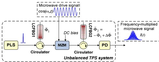
Figure 4. Schematic diagram showing an unbalanced temporal Fourier transform pulse shaping system for microwave waveform generation. PLS: pulsed laser source, LCFBG: linearly chirped fiber Bragg grating, MZM: Mach-Zehnder modulator, PD: photodetector, TPS: temporal pulse shaping.
