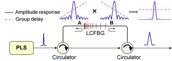
Figure 5. Schematic diagram showing the simplified frequency-domain Fourier transform optical pulse shaping system using a single LCFBG. PLS: pulsed laser source, LCFBG: linearly chirped fiber Bragg grating.
