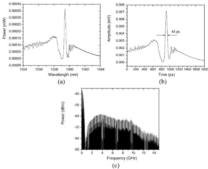
Fig. 3. UWB doublet pulse generation. (a) Spectrum after spectral shaping. (b) UWB doublet pulse. (c) Power spectrum of the generated UWB doublet.
