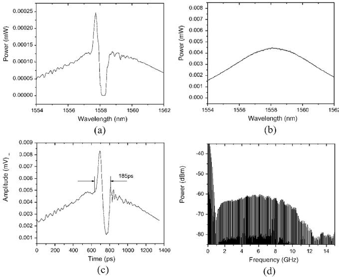
Fig. 2. UWB monocycle pulse generation. (a) Spectrum after spectral shaping. (b) Spectrum of the incident ultrashort pulse. (c) Generated UWB pulse. (d) Power spectrum of the generated monocycle pulse.
