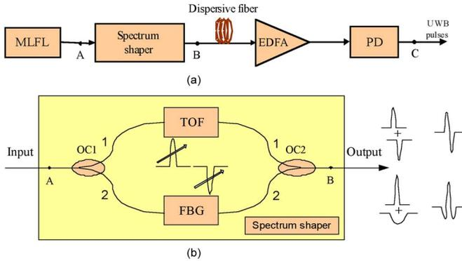
Fig. 1. (a) Block diagram of the proposed all-fiber UWB signal generation system. (b) All-fiber spectrum shaper configuration. EDFA: erbium-doped fiber amplifier. OC: optical coupler.
