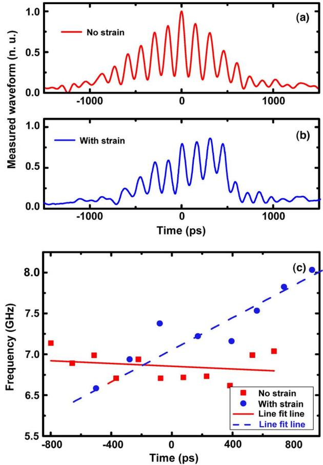
Fig. 7. Measured microwave waveforms: (a) with no strain, (b) with strain, and (c) the corresponding frequency chirps with and without mechanical force applied to the free end of the cantilever beam.
