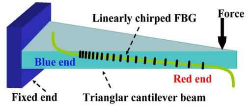
Fig. 5. Schematic showing the tuning the TOD of an NL-CFBG using the strain-gradient beam-tuning technique.
