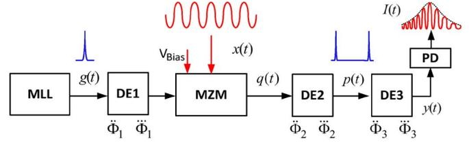
Fig. 1. Schematic showing the proposed unbalanced TPS system for chirped microwave pulse generation. MLL: mode-locked laser; DE1: the first dispersive element; MZM: Mach–Zehnder modulator; DE2: the second dispersive element; DE3: the third dispersive element; PD: photodetector.
