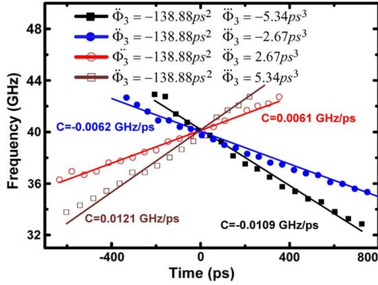
Fig. 3. Frequency chirps corresponding to the generated chirped microwave waveforms shown in Fig. 2.
