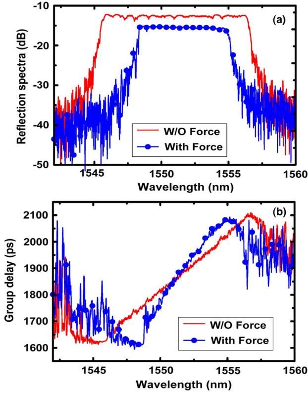
Fig. 6. (a) Reflection spectra and (b) group delay responses of the NLC-FBG with and without mechanical force applied to the free end of the cantilever beam.
