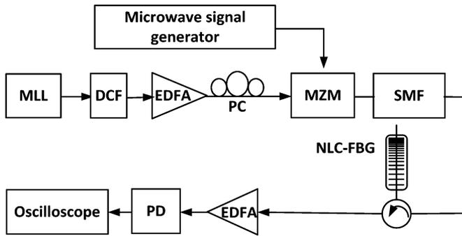
Fig. 4. Experimental setup. MLL: mode-locked laser; DCF: dispersion compensating fiber; EDFA: erbium-doped fiber amplifier; PC: polarization controller; MZM: Mach-Zehnder modulator; NLC-FBG: nonlinearly chirped fiber Bragg grating; SMF: single-mode fiber; PD: photodetector.
