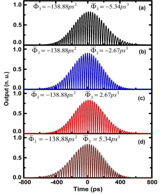
Fig. 2. Simulation results for the generated chirped microwave waveforms based on the proposed unbalanced TPS system with the third dispersive element having different TOD.
