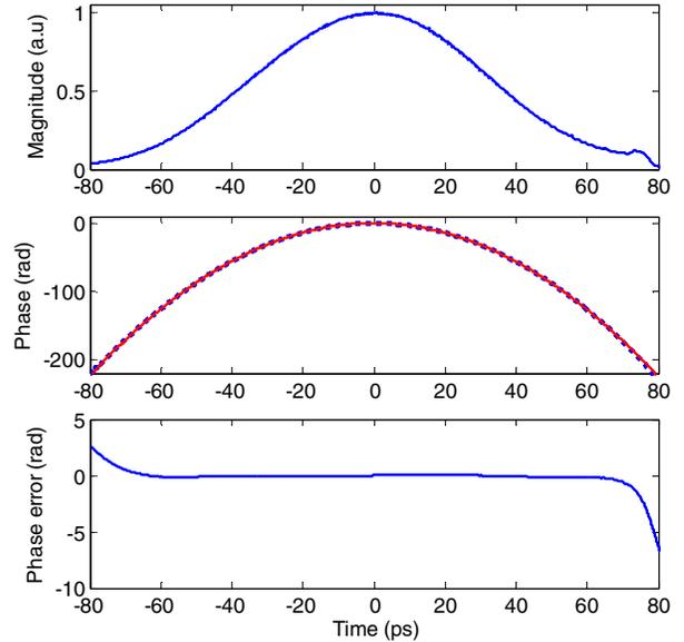
Figure 4. Reconstructed (a) temporal magnitude and (b) temporal phase of the PUT, calculated by the Fourier transform of Fig. (3) (Dashed line: measured phase, solid line: calculated phase). (c) Temporal phase measurement error.
