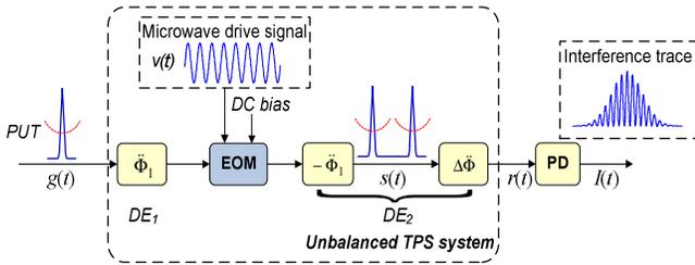
Figure 1. Schematic of the proposed pulse characterization system. PUT: pulse under test; DE: dispersion element; EOM: electro-optic modulator; PD: photodetector.
