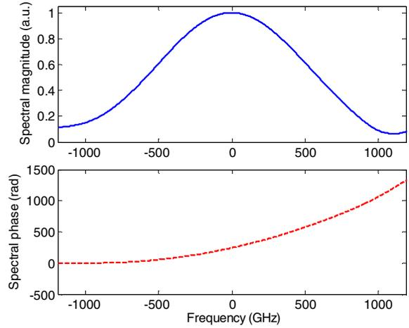
Figure 3. (a) Spectral magnitude and (b) spectral phase of the PUT, reconstructed from the measured temporal interferogram.
