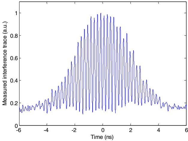
Figure 2. Measured interference pattern between two stretched and time-delayed replicas of the PUT using a real-time oscilloscope.
