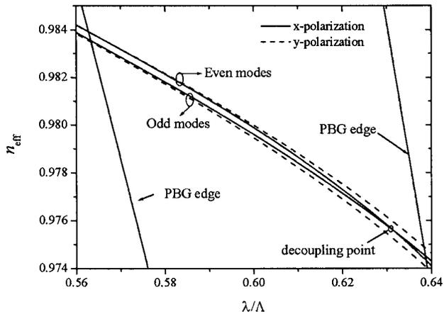
Fig. 2. Effective index of the PBG edges and the defect mode in a dual-core PBGF.
