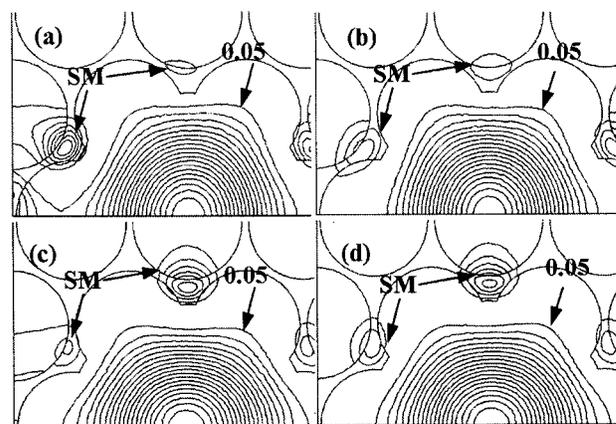
Fig. 4. Intensity contour maps of a one-quarter structure (a) even mode for  $x$  polarization, (b) odd mode for  $x$  polarization, (c) even mode for  $y$  polarization, (d) odd mode for  $y$  polarization at decoupling wavelength  $\lambda = 0.632\Lambda$ . The surface modes (SMs) are marked. Each contour is a 0.05 step from 0.05 to 0.95.
