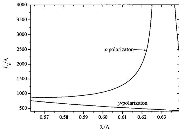
Fig. 3. Normalized coupling length of a dual-core PBGF. (The value over 4000 is not shown.)
