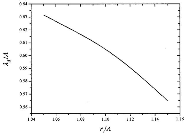
Fig. 5. Normalized decoupling wavelength  $\lambda_d/\Lambda$  as a function of normalized core radius  $r_c/\Lambda$ .
