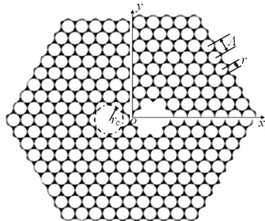
Fig. 1. Cross section of dual-core PBGF. One-quarter of the structure is considered in the FEM simulation.
