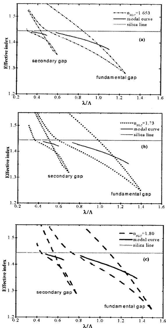
Fig. 3. Modal dispersion curve versus normalized wavelength when the refractive index of the NLC for  $y$ -polarized light is (a) 1.635 (b) 1.73, and (c) 1.80.
