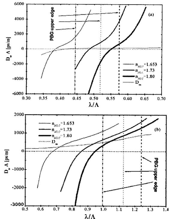
Fig. 6. Normalized GVD versus normalized wavelength with different refractive index of NLC when the refractive index of NLC for  $y$ -polarized light is 1.635, 1.73, and 1.80; (a) secondary gap region, (b) fundamental gap region.
