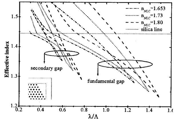
Fig. 2. Bandgap map of the NLC-filled MF versus normalized wavelength when the refractive index of the NLC for  $y$ -polarized light is 1.635, 1.73, and 1.80.
