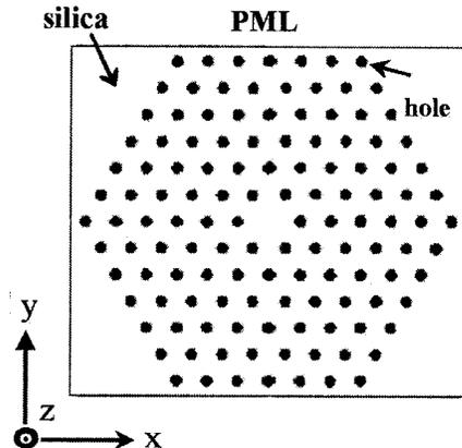
Fig. 1. Cross section of the microstructure fiber.
