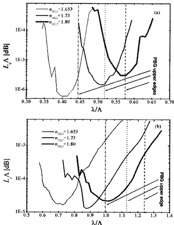
Fig. 5. Normalized leakage loss versus normalized wavelength with a different refractive index of the NLC when the refractive index of the NLC for  $y$ -polarized light is 1.635, 1.73, and 1.80; (a) secondary gap region, (b) fundamental gap region.
