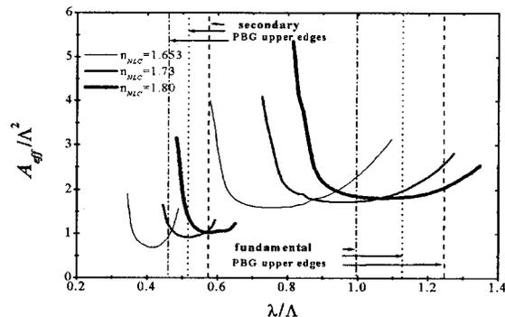
Fig. 4. Normalized effective mode area as function of normalized wavelength when the refractive index of the NLC for  $y$ -polarized light is 1.635, 1.73, 1.80.
