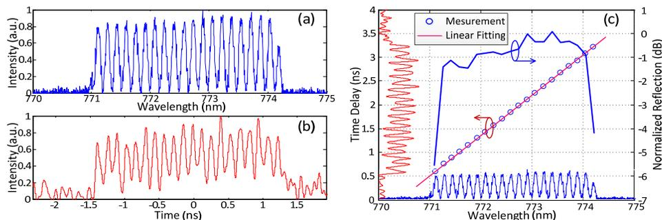
Fig. 2. Experimental demonstration of dispersive Fourier transformation near  $\sim 800$  nm using a chirped fiber Bragg grating. (a) Spectral fringe pattern measured by a conventional optical spectrum analyzer; (b) Temporal waveform measured by the photodetector and displayed on the real-time oscilloscope; (c) Time delay response and normalized reflectivity of the 800-nm chirped fiber Bragg grating.
