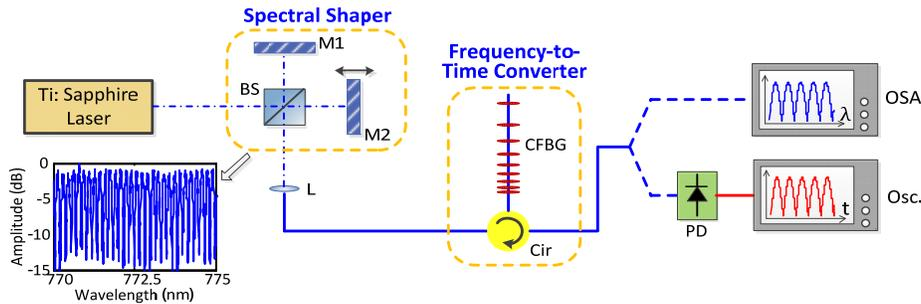
Fig. 1. Experimental setup for dispersive Fourier transformation near 800 nm (BS = beam splitter, M = mirror, L = lens, Cir = circulator, CFBG = chirped fiber Bragg grating, PD = photodetector, OSA = optical spectrum analyzer, Osc = oscilloscope). The inset shows the measured spectral response of the Michelson interferometer.
