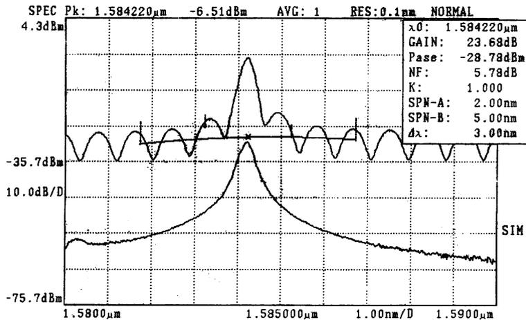
Fig. 4. Typical gain measurement spectra with input signal power of -30 dBm.
