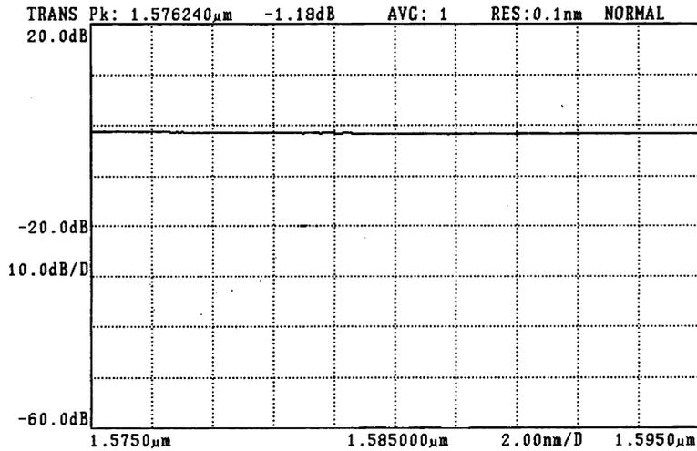
Fig. 5. Reflection spectrum of conventional 3 dB fiber loop mirror.
