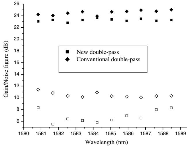
Fig. 3. Gain (shaded) and noise figure (clear) as functions of input signal wavelength.
