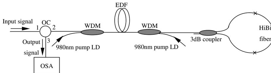
Fig. 1. Experimental setup of the noise figure improved EDFA based on ASE rejection technique.
