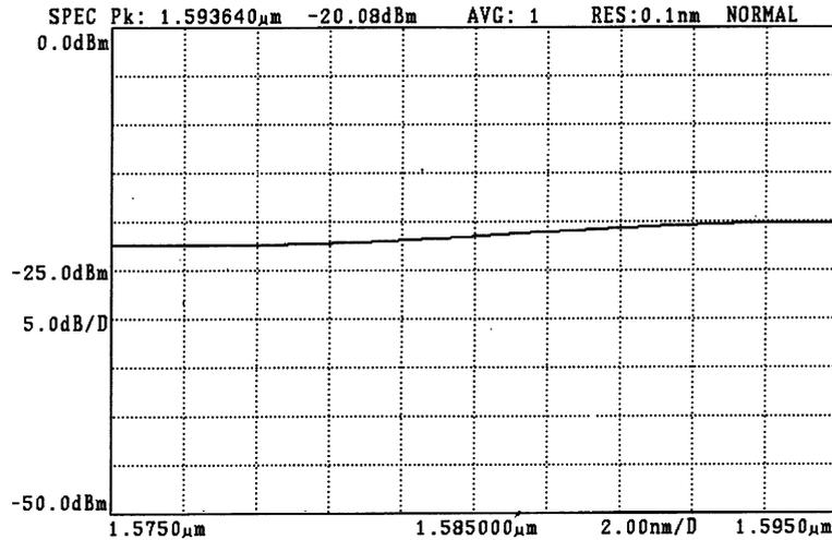
Fig. 7. Output spectrum of the conventional double-pass amplifier based on 3 dB fiber loop mirror.
