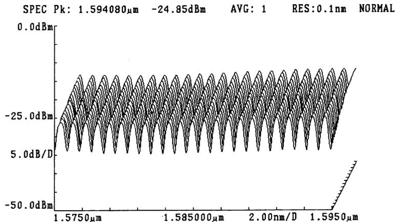
Fig. 6. 16-times repeated scans of the double-pass amplifier output spectra based on HiBi fiber loop mirror.
