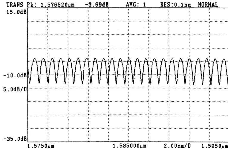
Fig. 2. Reflection spectrum of the HiBi fiber loop mirror.
