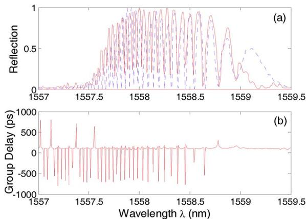
Fig. 2. (a) Measured (solid line) and the simulated (dashed line) reflection spectra and, (b) reflection group delay of the SI-CFBG.
