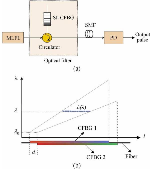
Fig. 1. (a) Schematic diagram of proposed electrical chirped pulse generation system. (b) SI-CFBG-based chirped FSR optical spectral filter.
