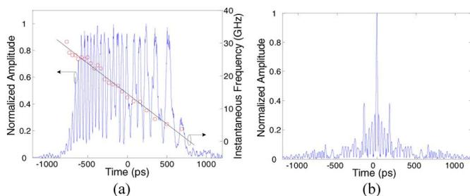
Fig. 3. (a) Measured pulse profile and instantaneous frequency of the generated chirped microwave pulse. (b) Autocorrelation waveform of the generated chirped microwave pulse.
