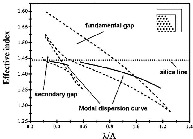
Fig. 2. Modal dispersion curve for the fundamental mode of NLC-filled MFs as a function of normalized wavelength.
