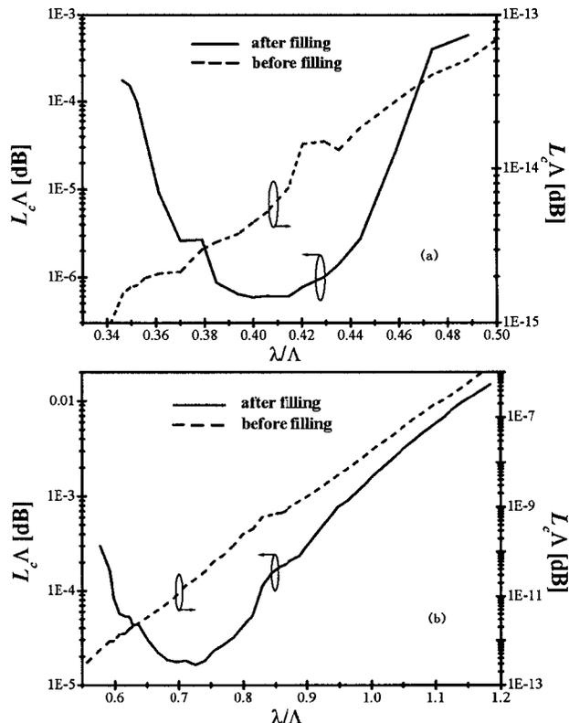
Fig. 4. Normalized leakage losses of the fundamental mode as a function of normalized wavelength in the (a) secondary and (b) fundamental gap regions of the MFs before and after filling them with NLC.
