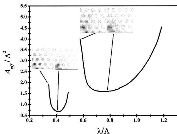
Fig. 3. Normalized effective mode area for the fundamental mode of NLC-filled MFs as a function of normalized wavelength.
