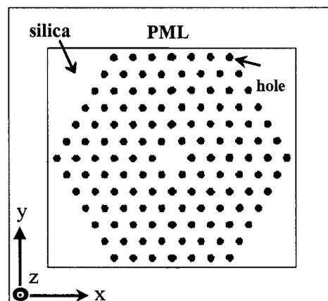
Fig. 1. Cross section of the microstructure fiber.
