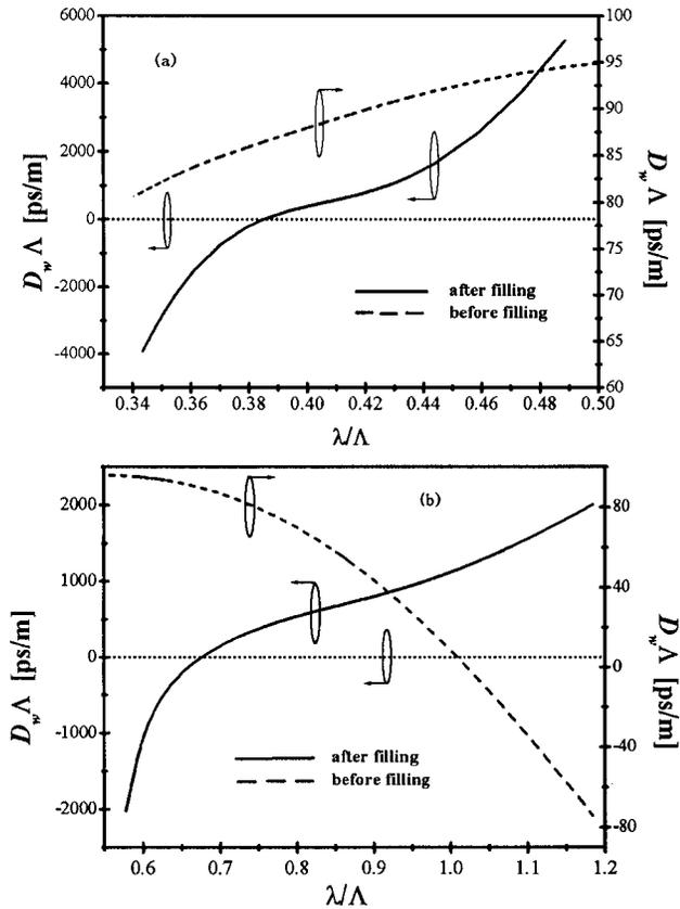
Fig. 5. Normalized GVD of the fundamental mode as a function of normalized wavelength in the (a) secondary and (b) fundamental gap regions of the MFs before and after filling them with NLC.
